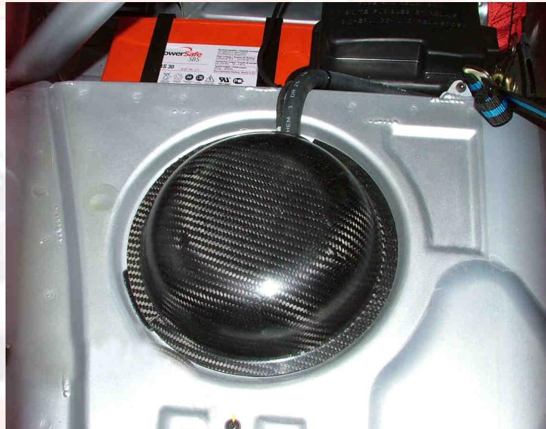
Fit a panel grommet ([ref. 8](#)) on the vent hose ([ref. 1](#)), and screw this on the filler plate, as shown in the photo opposite.
