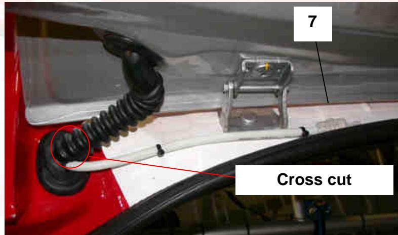
Attach the check valve to the rear wing liner using a rilsan (by the cut-out at that location).
